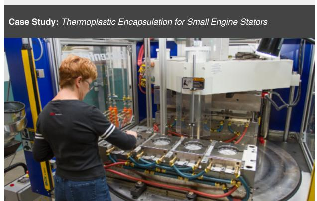
Thermoplastic encapsulation, a custom injection molding technique used by Plastic Parts, Inc. is utilized to develop cutting-edge stators for Briggs and Stratton Corporation, maker of small engines for outdoor power equipment. The redesigned stators deliver the benefits of improved protection against heat and moisture, higher manufacturing yields and lower production costs.
