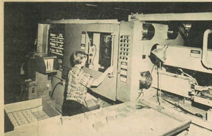
(Union Grove)—Diane Anderson, Racine, is operating the large 350 ton Lester injection molding machine as molds are made for a new style of children's building blocks. The blocks will go to a manufacturer of children's toys for completion.
